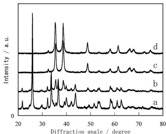
Fig. 4. XRD patterns of microwave irradiated specimen for (a) 0 min, (b) 10 min, (c) 30 min and (d) 60 min at 95 °C.
