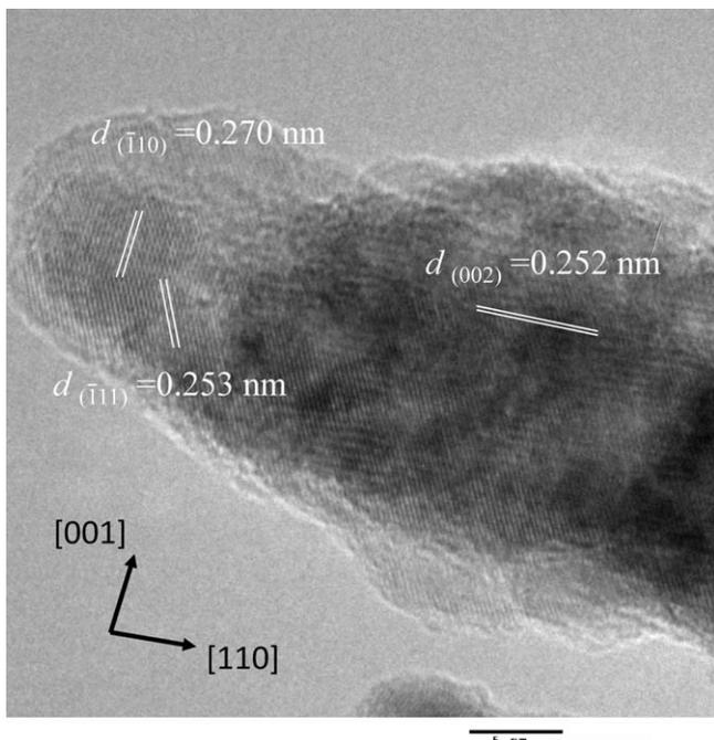
Fig. 7.  $[-1\ 1\ 0]$  projection of HRTEM image for CuO microcrystal synthesized by microwave irradiation.
