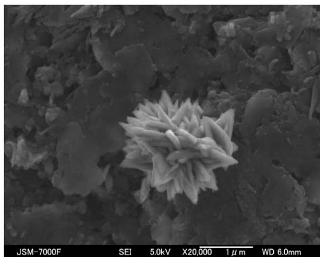
Fig. 5. SEM images of the synthesized CuO microcrystals using (a) mantle heater and (b) microwave irradiation.
