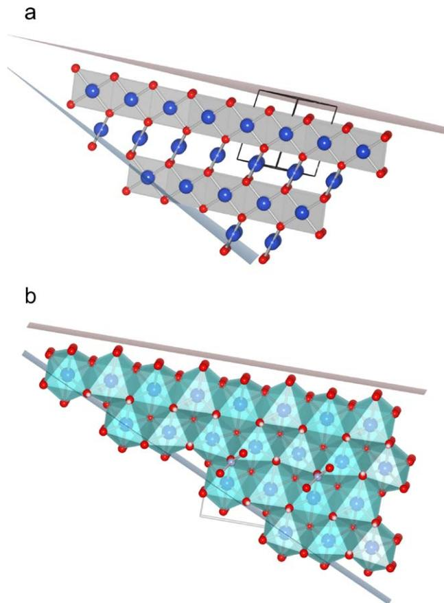
Fig. 8. Schematic drawings of a crystal directions for (a) the monoclinic CuO corresponding to Fig. 7 and (b) the copper precursor that corresponding to the same position.
