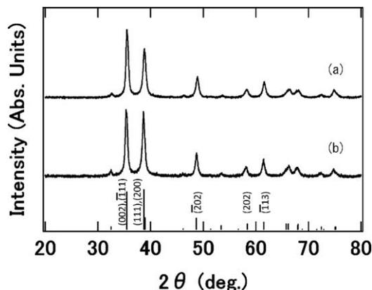
Fig. 3. XRD patterns of the synthesized CuO microcrystals using (a) mantle heater and (b) microwave irradiation.
